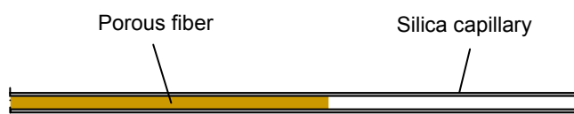
Figure 6 Schematic of the CEC column consisted of the polymeric porous full fiber inside a silica capillary
